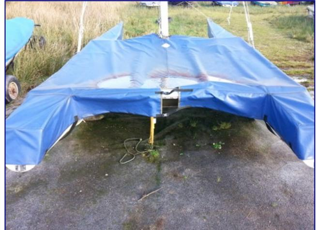
In the picture on the left, the rear tie down passing over the cover would be better passed under the cover so that the tie down rope can be kept tight whilst allowing the cover to be raised to let the water drain off.
